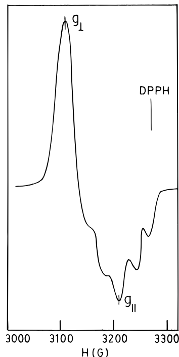
Figure 2. X-band EPR spectrum of [Ni(Ph 3 L)]PF 6 in frozen 1:1 acetonitrile–toluene solution at 77 K.
